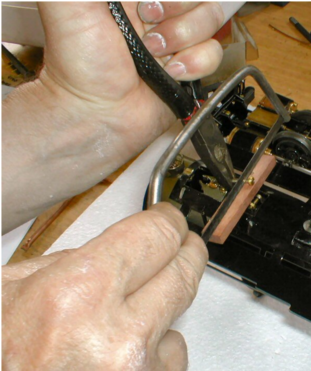
FIG 8. Cutting the end off the steam pipe.
