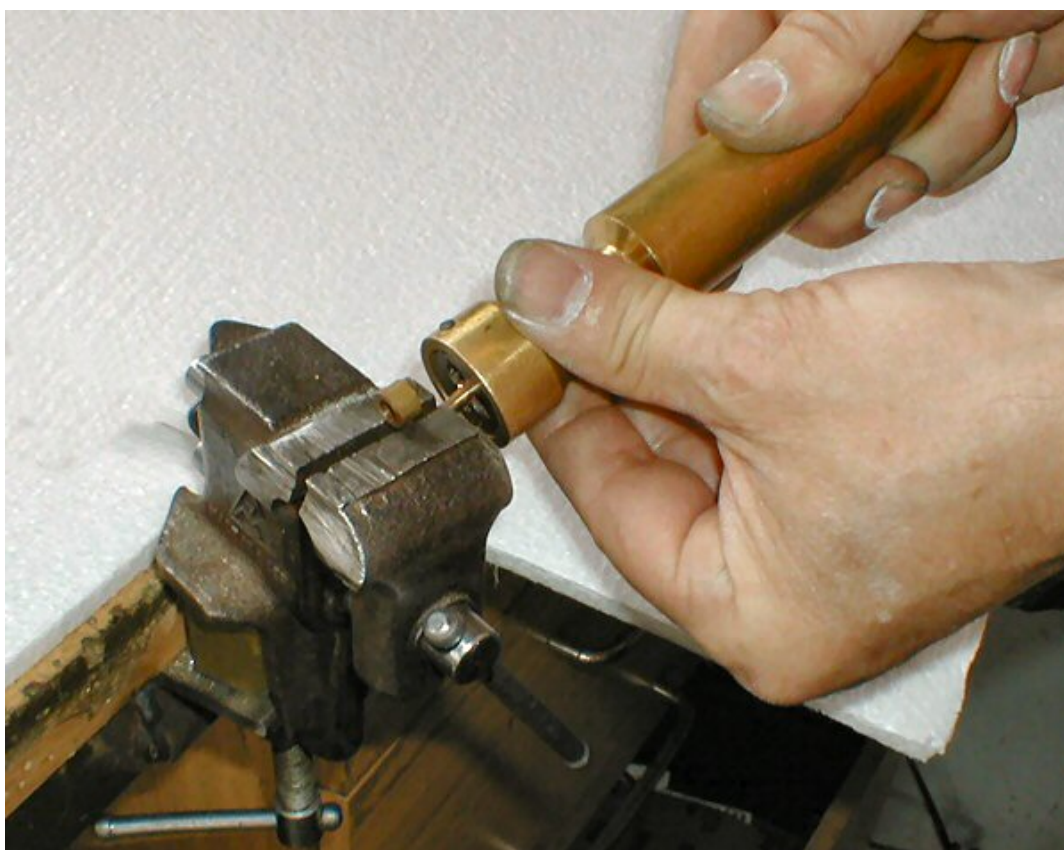
FIG 12. Threading the end off the copper pipe.
