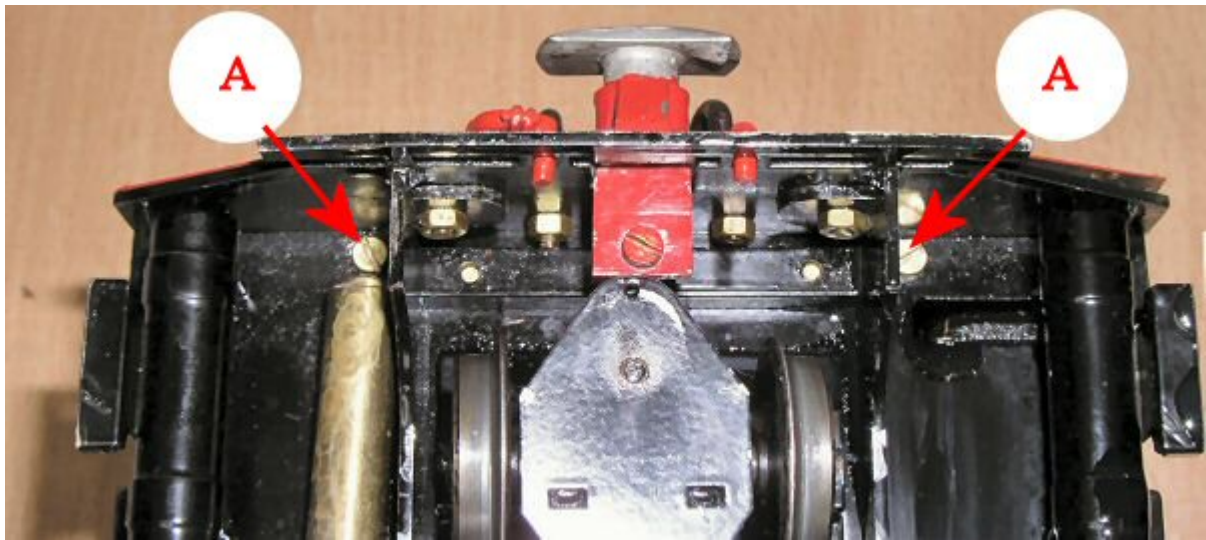
FIG 3. Rear cab fixing screws.
